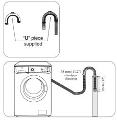
Firstly form a hook in the end of the drain hose using the «U» piece supplied. Place the drain hose into your standpipe, which should have an internal diameter of approximately 38mm thus ensuring there is an air break between the drain hose and standpipe. When discharging into a standpipe ensure that the top of the standpipe is no more than 90 cm (35.4") and no less than 60 cm (23.6") above floor level.
